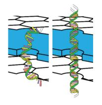
Graphene-DNA hydrophobic interactions slow DNA transport through a nanopore. The introduction of graphene layers makes the pore and membrane surface hydrophobic, leading to sticking interactions with the ssDNA molecules. On the other hand, dsDNA has far less significant hydrophobic interactions with graphene as nucleobases are shielded in the helical structure.
