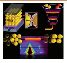
Inorganic treatment of nanocrystals removes traps, increases long-range ordering of the symmetry, and improves stability in solar cells. A combination of optical, electronic, and material characterization tools demonstrates that chloride treatment confers many benefits on photovoltaic materials.
