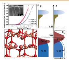
$Cu_2O_{1-\delta}$  (111) exhibits promising field emission properties with interesting electron tunneling behavior at low turn-on and threshold voltages of 0.8 and 2.4 V  $\mu m^{-1}$ respectively. Density functional theory suggests that oxygen vacancies enhance the electron donating ability because of unshared d-electrons of Cu atoms (nearest to the vacancy site), allowing an impurity energy state  $(E_{im})$  close to the conduction band.
