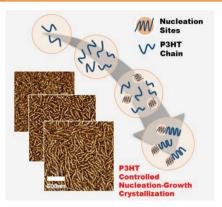
Mechanistic elucidation of P3HT molecular assembly is presented based on the experimental demonstration of controlled P3HT nanorod fabrication. The 2-step crystallization model comprises nucleation and growth steps, and is successfully adopted to interpret P3HT assembly into mesoscale entities. Systematic control of nucleation and growth allows formation of P3HT nanostructures exhibiting enhanced charge transport performance.
