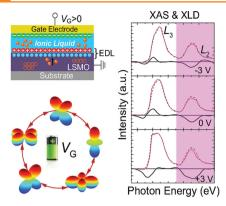
The orbital occupancy and magnetic anisotropy of (La,Sr)MnO3 films are manipulated by gate voltage in a reversible and quantitative manner, accompanied with the electronic phase transition. Positive and negative gate voltage increases and reduces the occupancy of the orbital and magnetic anisotropy that are initially favored by strain (irrespective of tensile and compressive), respectively.
